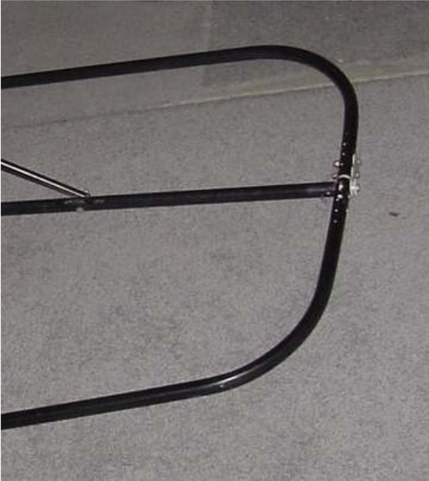
21. Once this stabilizer and elevator assembly is built you can mount it on the airframe. Verify that all the components are level and square with the boom tube / rudder, etc... after mounting on the airframe.
