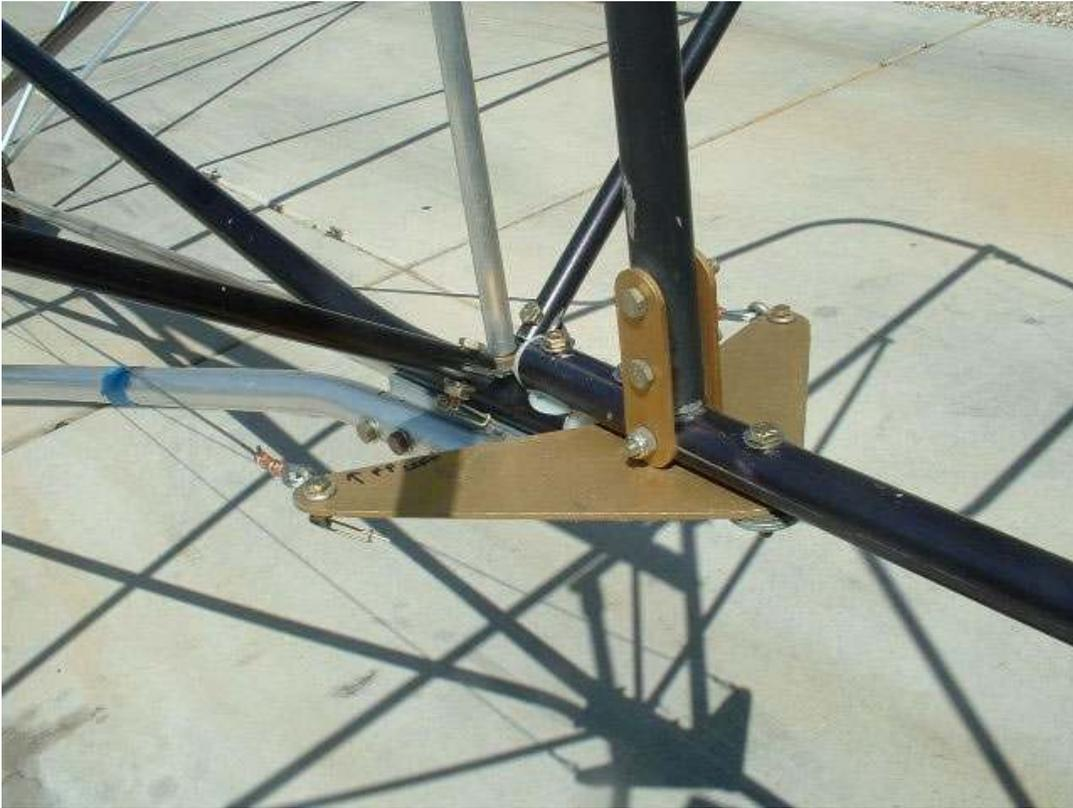
19. **Rudder:** Build the rudder parts: including the rudder horn, tangs, and rudder hinge bracket – assemble the tubing and mount it to the airframe. Should look similar to the photo above. You can support the rear of the airframe with a simple setup now as it is probably tail heavy and needs something to support it.
