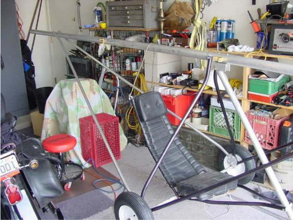
15. **Motor Mount:** If you have the motor for your plane I suggest that you build the motor mount, get it mounted. This is required on some setups to mount the front fuse tubes to a mount point that is part of the engine mounting system.
